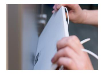
The keyboard can also be attached to almost any magnetic surface at an angle of up to 90° from horizontal as a result of its in-built magnets. An integrated capacitive touchpad handles the mouse functions. The divided space bar and the gentle, but precise key strokes provide a pleasant feel for people using the unit and support touch-typing.
