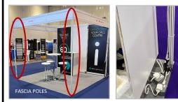
Shell Scheme stands have Nameboard Fascia support poles to the front. The Fascia structure can be used to distribute power from the stand back wall, overhead to the front pole. \*Stands with over 4m open side have corner and central fascia support poles
