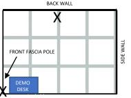
Example Socket Position Diagram 4m x 3m 2 Open Sides X = Socket Positions - to back wall and fascia pole 1 Square = 1m
