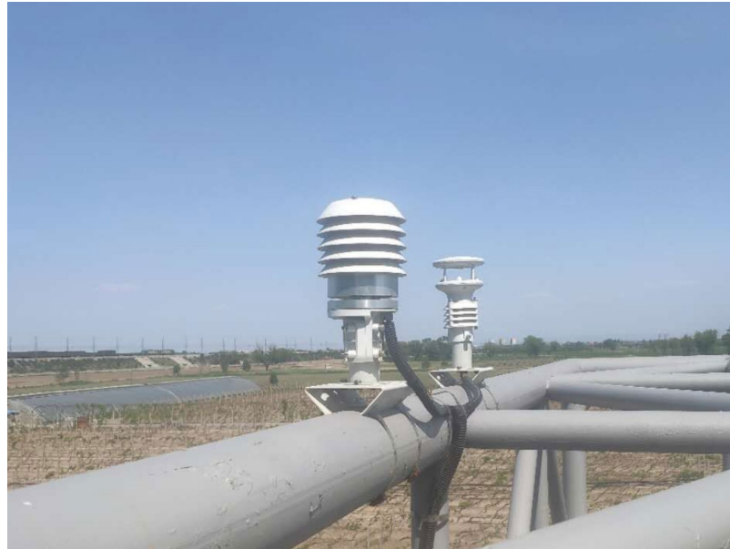
Air quality and weather sensors in farm
