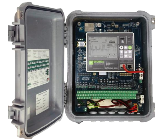
METEODATA-4016CP COMPACT POLYPROPYLENE IP67 CABINET 34 x 29.5 x 15.2 cm
