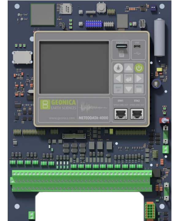
METEODATA-4000 Main Board with HMI-4000 Graphical Display
