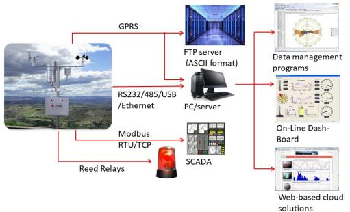
Name is known for the flexibility of its signal acquisition and data processing system. Produced data is then processed by LSI LASTEM or third-party applications.
