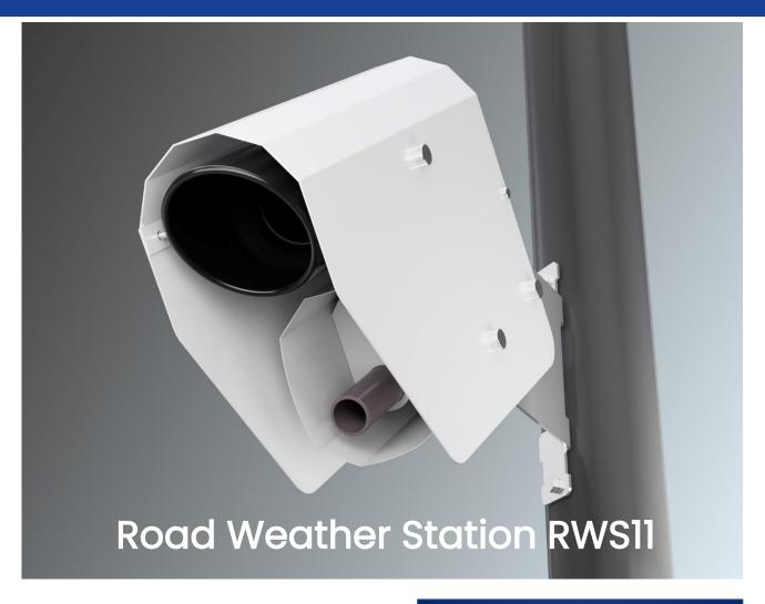
Road Weather Station RWS11 is a compact station for all basic road weather measurements. The station is designed for use as an optimization tool for winter maintenance. RWS11 is also suitable for runway condition reporting. The station can be installed onto an existing pole along the roadside to follow surface conditions and friction in real time.
