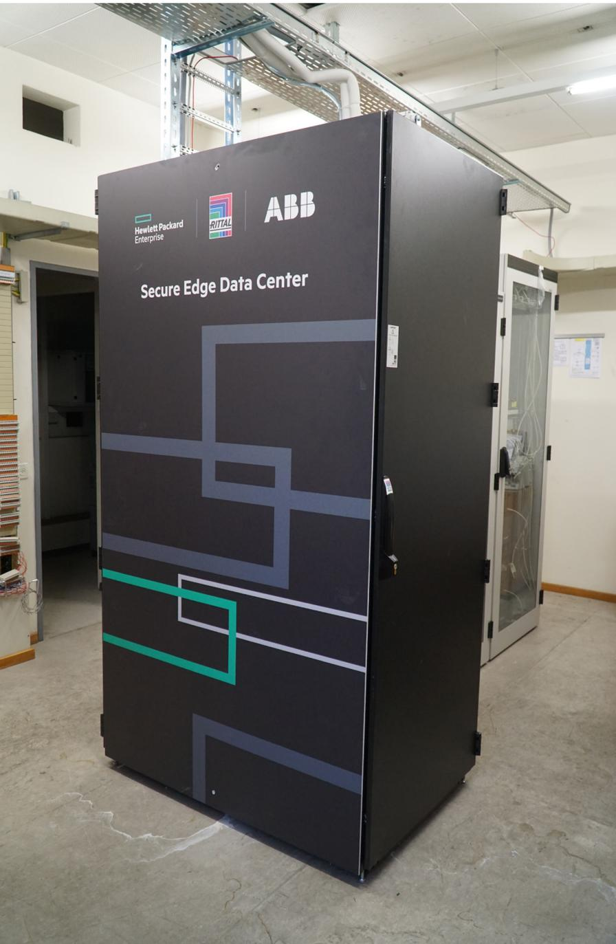
The Secure Edge Data Center (SEDC) is an all-in-one plug and play industrial data center solution that is specifically designed to run in industrial environments, bringing enterprise-grade IT capacity closer to the point of data collection and machine control.
