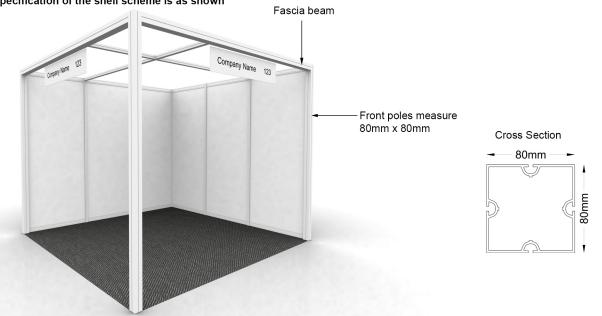
990mm centres between posts 990mm centres between posts Seen size Seen size 950mm x 2340mm Cut size Cut size 964mm x 2354mm 944mm x 2354mm 80mm x 80mm 930mm between Posts 950mm between Posts
