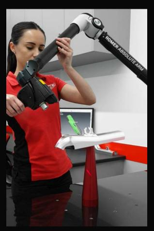
The software has the capability of importing a nominal model and comparing the measured data deviation.
