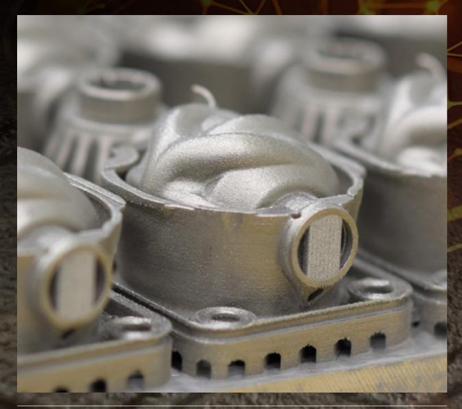
Despite the potential of AM, it had traditionally been limited to low-volume custom applications in aerospace, medical, and automotive industries. Domin desired a platform that could make AM more viable for high-volume production, and the four 500W lasers in the RenAM 500Q provided the significantly higher build rates, part quality and competitive machine costs needed for their application.
