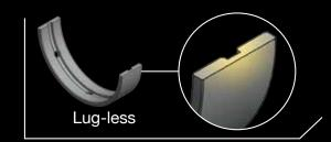
For aftermarket installers, placing a lug-less bearing into its correct position requires additional accuracy and attention to details. Shell and housing should be aligned for unimpeded oil hole orientation and for proper centering to avoid bearing-to-crank fillet ride.
