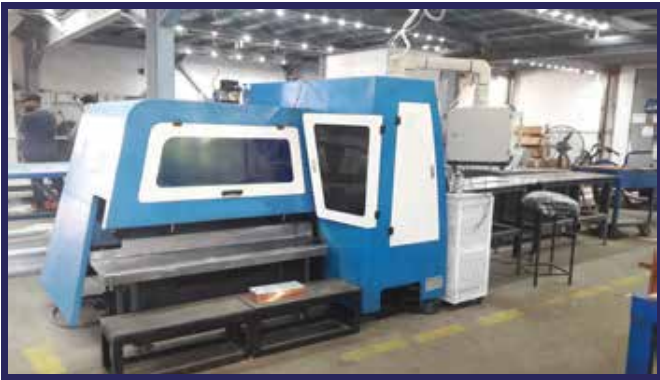
Two CNC Machines for Conductor Cutting & Punching
