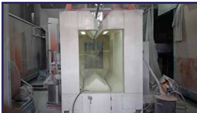
Automated Electrostatic Painting Line Will be upgraded to be 20 automated gun and 4 manual guns
