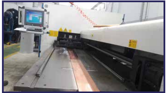
Two CNC Machine for Conductor Cutting, Punching & Forming
