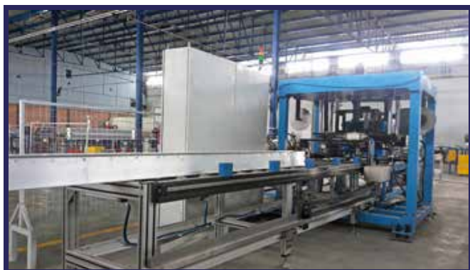
Four Automated SPR Machine SPR Self Piercing Riveting
