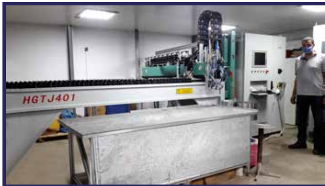
One State of the Art CNC FIPFG Machines FIPFG Formed In Place Foam Gasket
