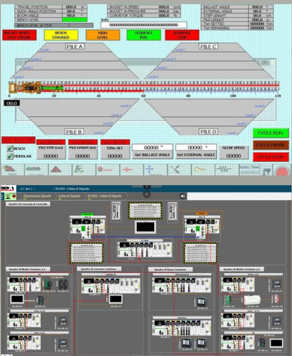
Running an automated system requires creating an operator interface to oversee line activities and activate the various planned processes. A plant supervision system, based on a PC, Panel PC or Operator Panel, makes it possible to view the layout and P&I of the system in real time, along with statuses, alarms, and data that update continuously on the line.
