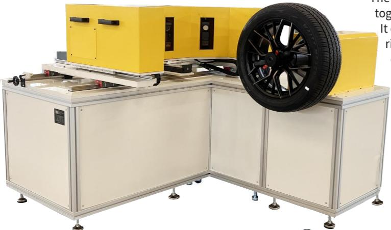
The tire profile measurement and analysis system is a non-contact 3D scanning system composed of a stable, precise mechanical structure and line laser sensors. The system utilizes multiple line laser sensors working together to capture the tire's profile and record test data. It can measure not only the external profile of the tire rim but also analyze tire geometry and wear, among other aspects.
