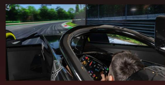
**Fine Adjustments:** pedals and seat are adjustable to accommodate people of virtually all sizes and ages, allowing the driver to assume the typical lying position of a Formula 1 driver.
