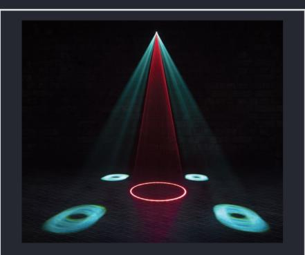
Being able to widen the size of the beam means that it is possible, to some extent, to replicate the primary effect of moving heads, making BeamBrush laser projectors more flexible and very useful for lighting designers. And, let's not forget about the advantages of a wider beam regarding laser safety!
