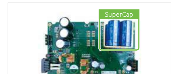
Protection for voltage dips
