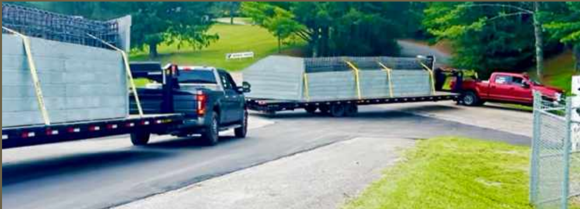
3 Lightweight components, easily transported by small trucks
