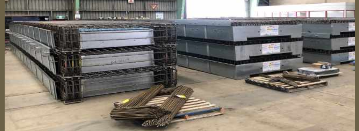
2 Modular units are easily stacked and stored for quick delivery
