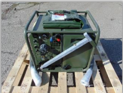
Variable Tactical Electrical Generator (VTEG) 6.5 kW
