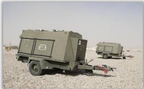
Field Electrical Power Source (FEPS) 20-40 kW
