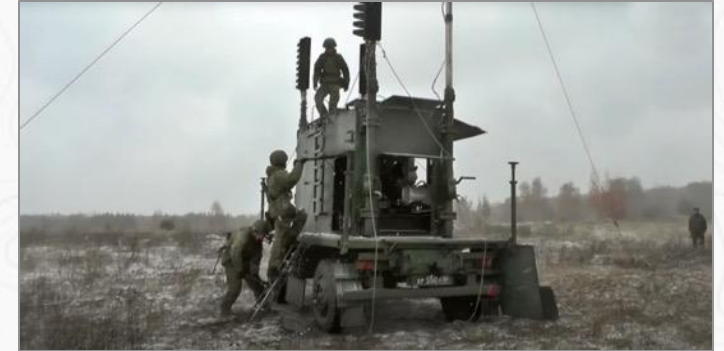
The Russian R-330Zh Zhitel EW jamming system can shut down, over tens of kilometers, GPS and satellite communications. This image shows the base of one of the four antennas in a typical setup.
