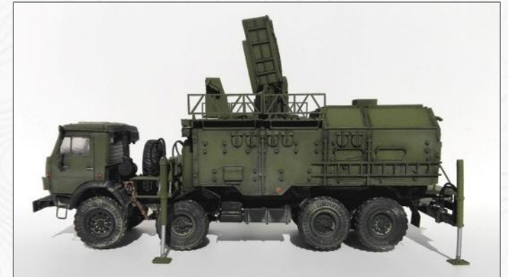
The Russian 1L265 Moskva-1 is a precision HF/VHF ES receiver that is used to passively detect and analyze an opponent's transmissions, such as that of drone operators.
