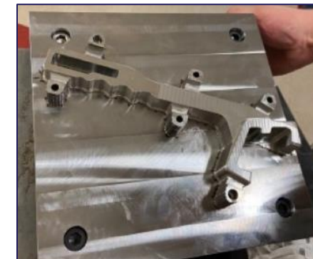
Fire Spanner Wrench Application Machining (first pass)
