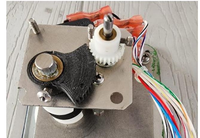
Value control part manufactured to execute required repair prior to underway
