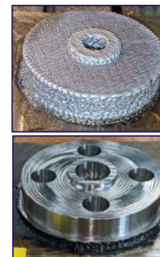
A/C Flange Application As-built near-net shape (top) Machined (bottom)
