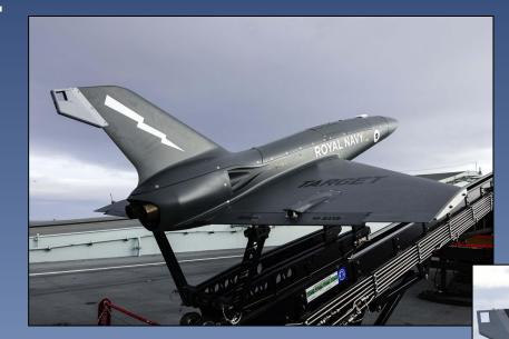
Project Vampire is a low cost fixed wing fast jet uncrewed air system which is part of a spiral development project within the Maritime Uncrewed Air Systems programme (MUASP). It is developing a deployable threat simulator for air defence training, and to provide a trial platform to practically deliver sensors and effectors, integration for the Naval Strike Network (NSN) and build evidence for Integrated Review (IR25).
