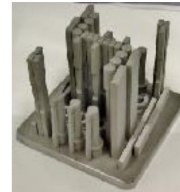
Example qualification build plate
