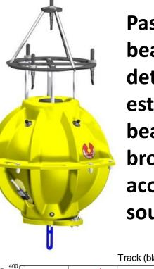
Passive bearing detector (PBD) establishes bearing to broadband acoustic source
