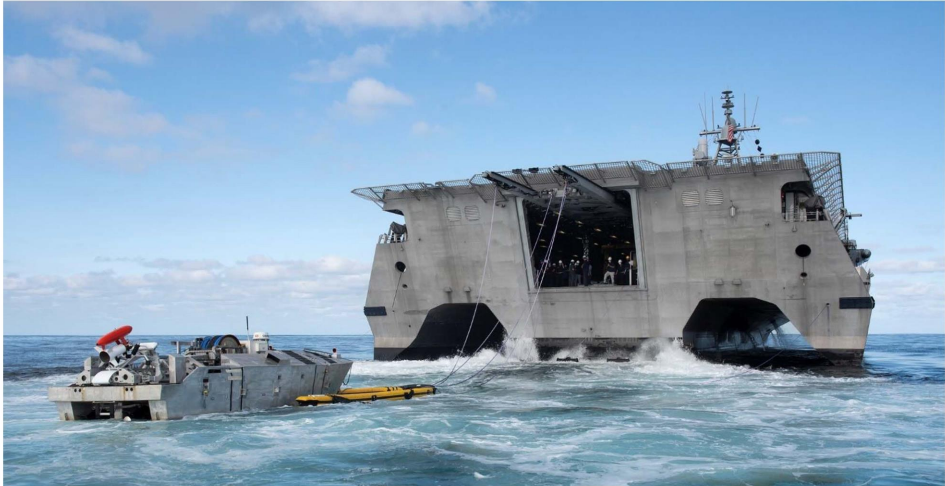
Shown: Magnetic and acoustic influence sweep systems on MCM USV (UISS) during launch/recovery operations behind an Independence-Class LCS
