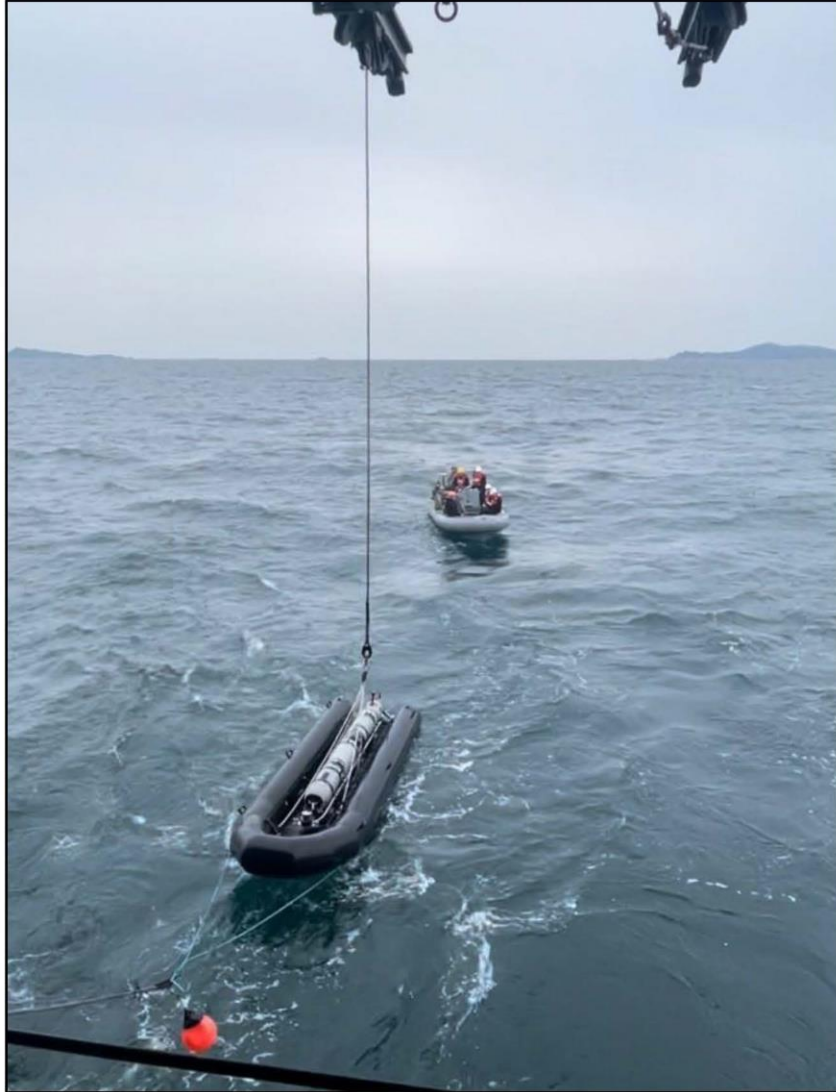
Shown: MK18 Mod 2 UUV launch and recovery operations from Independence-Class LCS
