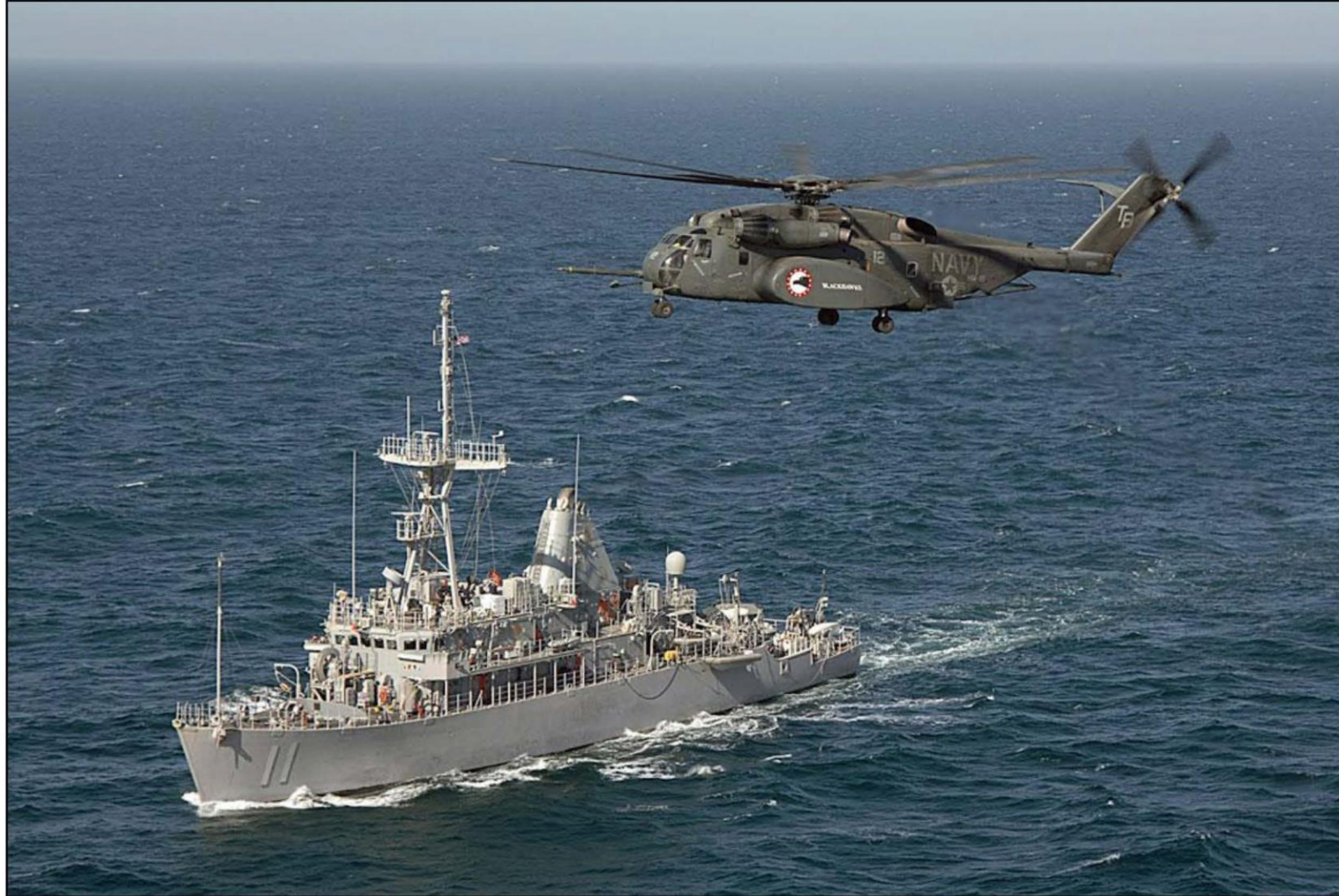
Shown: USS Gladiator (MCM-11), an Avenger Class MCM ship and MH-53, the Navy's primary aerial MCM aircraft
