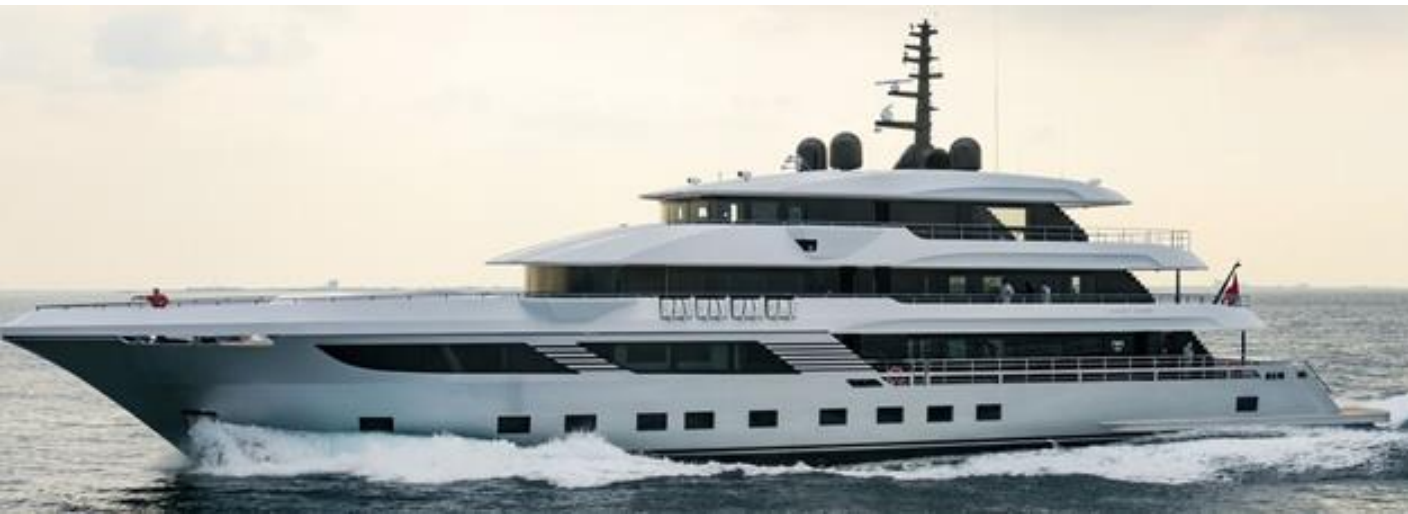
Majesty 175 world's largest composite production superyacht built from carbon fibre and vinylester.
