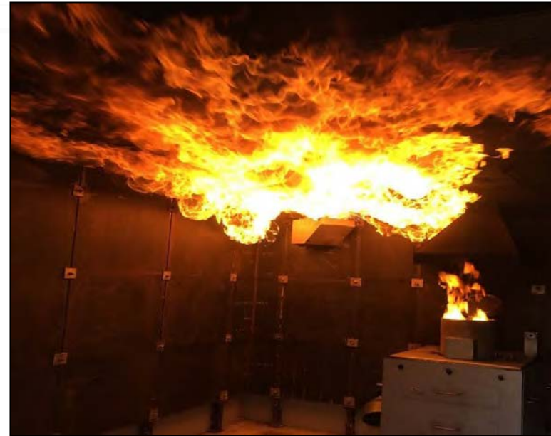
Galley Fire with Flashover
