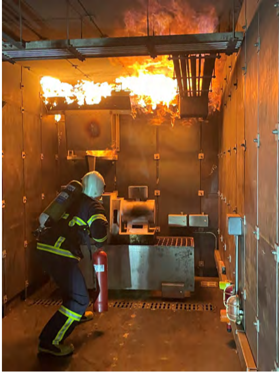
Electric Motor Fire Cable Tray Fire
