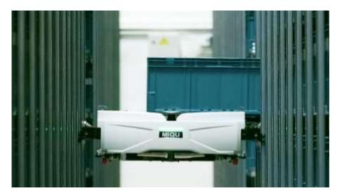
The Skypod is a robotic order-picking system that can also be used as a buffer solution for prepared orders. Upstream and downstream of the Skypod robot, Exotec is able to customize according to the level of automation, logistics characteristics and distribution channels of their customers. Exotec can support the growth of any activity without interrupting production by simply adding robots, stations or racks. The solution is simple and quick to set up.
