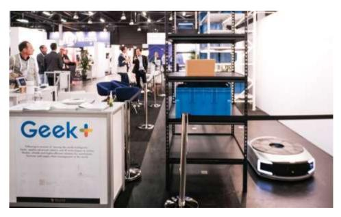
Geek+ attended DELIVER 2021 with their Robot Arm Hybrid, the integration of an AMR (autonomous mobile robot) and a robot arm using the Geek+ moving management system. It offers high efficiency, flexibility and agility, and enhances pick and place automation operations by replacing traditional AGV and conveyor lines to finish the last step for lading and production.
