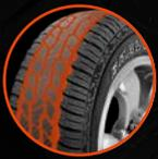
Four unique U-shaped circumferential grooves offer **excellent hydroplaning resistance** while **minimising rock retention**.
