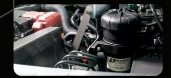
**Provent Ultimate Catch Can Kits** are designed to protect modern diesel engines from the harmful effects of blow-by gases. These gases, containing unburned fuel, oil mist, and soot particles, can accumulate in the intake system, leading to reduced performance, increased emissions, and potential engine damage. **The Provent Catch Can system effectively separates and captures 98% of these contaminants.**
