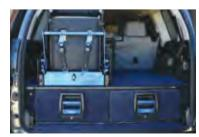
MSA 4X4's patented slide technology smoothly handles up to 250kg per pair of drawers providing smooth opening under heavy loads. A whole new level of access is provided to drawer contents, through the patented 2 stage over extension of the drawer for 100% easy access.
