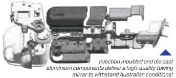
Designed to fold inwards or outwards when bumped in carparks or when in contact with trees and other obstacles around the vehicle.
