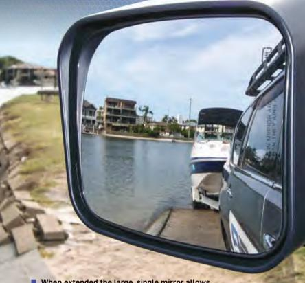
When extended the large, single mirror allows the driver to see beyond the caravan, trailer or boat and avoids the confusion of multi-lens mirrors for everyday driving.
