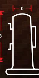
All measurements listed are measured on the internal surface of the turbo cover, so as to match the outside measurements of your turbo exhaust housing, please note that the turbo cover comes with spring mounting clips to give the cover a small amount of flexibility in fitment
