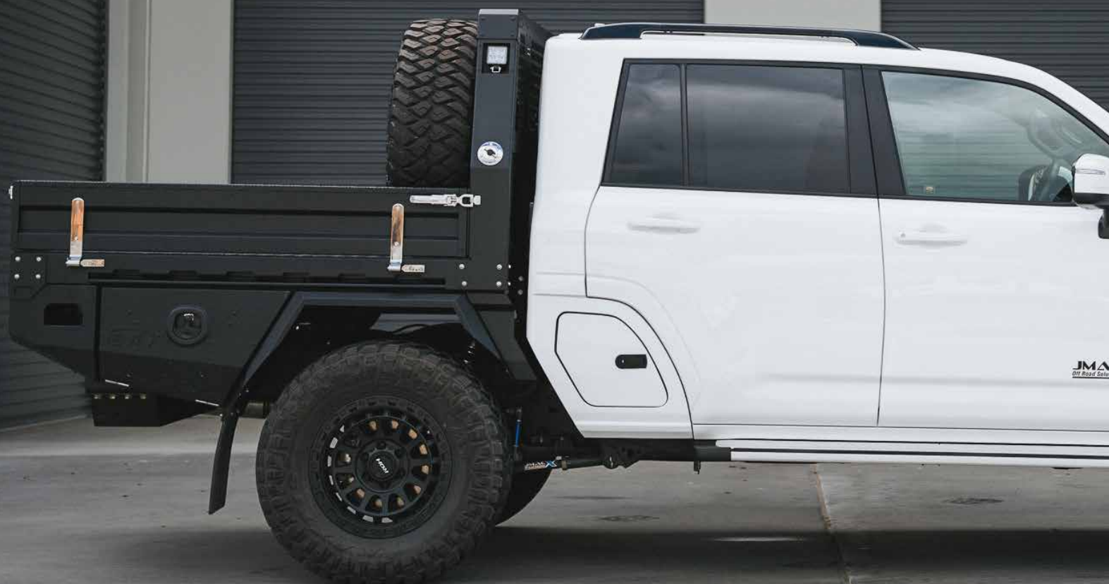
JMACX AEV LC300 W/600MM CHASSIS EXTENSION. TRAY: 1700L X 2000W
