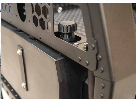
40L Headboard Water Tank
