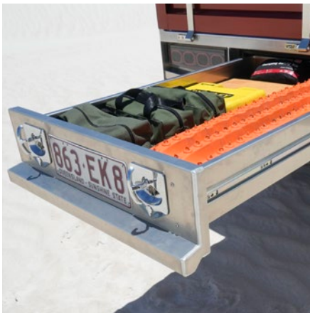
1200MM LONG REAR TRUNDLE DRAWER Store tools, shovels or spare parts in a 1200mm dust and water resistant trundle draw. Made with heavy-duty 227kg rated drawer slides.
