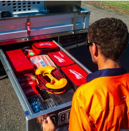
1600MM LONG LOCK OUT REAR TRUNDLE DRAWER Store tools, shovels or spare parts in a 1600mm dust and water resistant trundle draw. Made with heavy-duty 227kg rated drawer slides.
