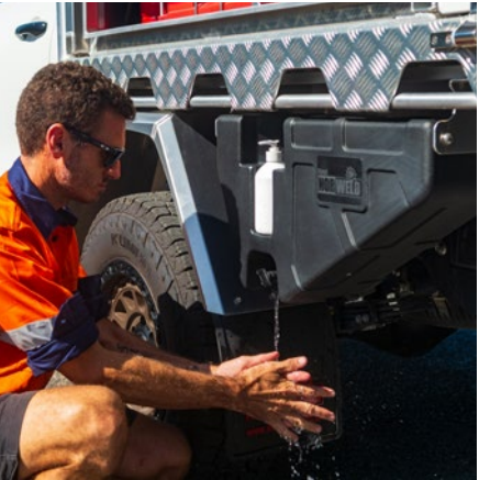
23L UNDER TRAY HAND WASH TANK 23L hand wash tank bolts under tray, allowing easy clean ups on site and between jobs. Includes soap dispenser.
