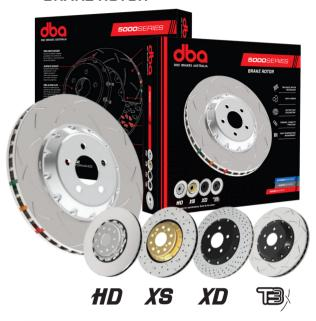
5000 SERIES high-performance rotors share all the benefits of the 4000 Series. They are a composite two-piece direct replacement brake rotor. We use only the highest quality materials to ensure optimal performance under the most strenuous circumstances, combining high carbon cast iron rings with aerospace grade aluminium hats (T6061-T6) held together with National Aerospace Standards (NAS) bolts and crimp nuts.
