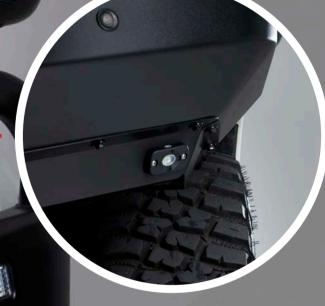
Optional directional lighting which can be ordered and fitted to the bar to replace the OEM light
