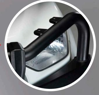
Three CB aerial mounts, ideal for UHF, Phone Aerial and Sand Flag - two located on the passenger side, one located on the driver's side – with each mount utilising a quick fit cut out so additional accessories can be easily installed later
