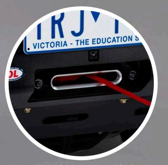
The location of the winch and fairlead has been designed with accessibility for when you need it most. The low winch mount allows for optimum vehicle recovery and is built to suit a wide range of popular winch models
