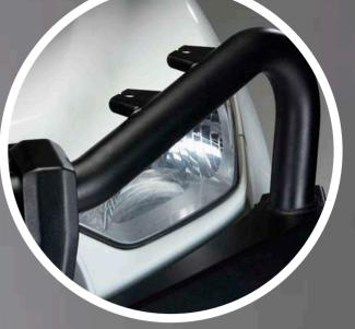
Three CB aerial mounts, ideal for UHF, Phone Aerial and Sand Flag - two located on the passenger side, one located on the driver's side – with each mount utilising a quick fit cut out so additional accessories can be easily installed later
