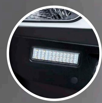
Recessed LED indicators are packaged with the bar and designed to reduce the risk of damage
