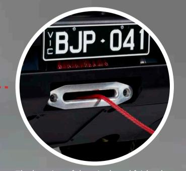
The location of the winch and fairlead has been designed with accessibility for when you need it most. The low winch mount allows for optimum vehicle recovery and is built to suit a wide range of popular winch models
