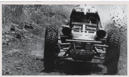
Mickey became known as the man who put big engines in off-road buggies. This is his V8 Chevy powered rear-engined buggy.
