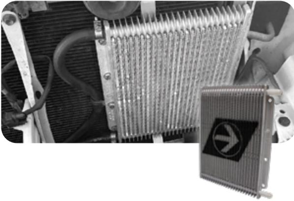
The Direction-Plus™ Transchill Transmission Oil Cooler kits are designed specifically to reduce excessive transmission heat caused by:
