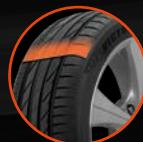
High performance polyester with very high denier in the body ply to **increase tensile strength and reduce weight**, produces **sharpened handling and steering response**.
