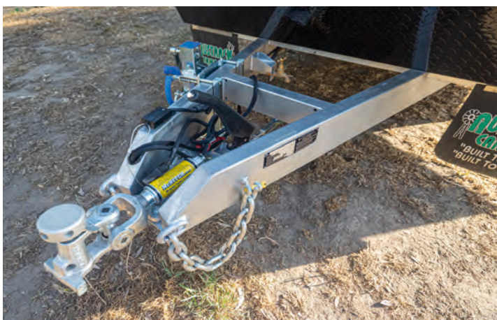
McHitch 3500 Kg uniglides platinum coupling with locking pin. Double ADR approved rated safety chains. Dual rear recovery points. Ark XO 750 Series extra heavy duty swing away dual wheel jockey wheel.
