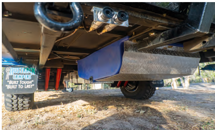
Water storage: 2 x 120L Foodgrade poly water tanks. 12.5L per min 12V Electric Pump. Water tank guards, water gauge.
