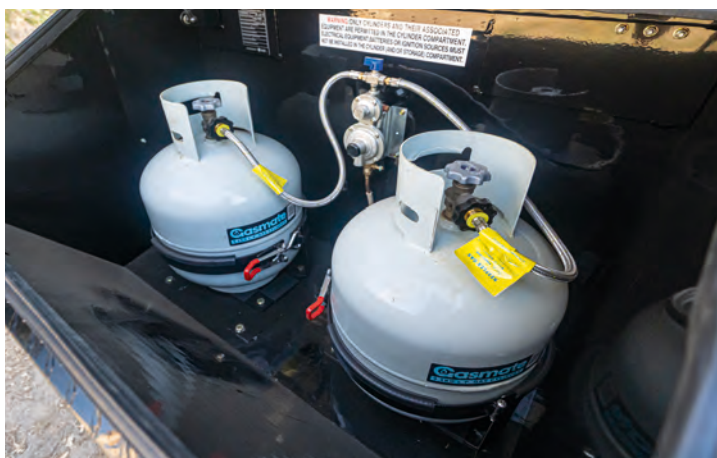
Completely plumbed from gas bottles to kitchen with dual bottle change over valve and gas certification certificate. Additional bayonet gas connection at rear of camper for a BBQ gas supply.
