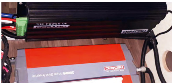
REDARC 2kW Pure Sinewave inverter with remote switch REDARC Manager30 complete battery management & charging system
