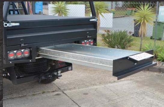
Rolla-drawer integrated into tail light panel
