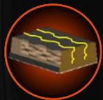
Closed-end bridging of sipes in the shoulder blocks ensure increased rigidity for a **stable drive**, and also help ensure **reduced noise generation.**
