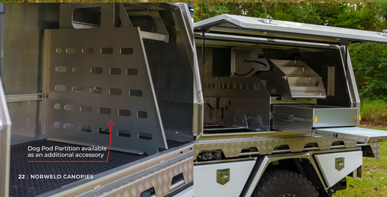
Norweld Deluxe Dog Pod Canopy (1900mm Length) | Full-Time Deluxe Canopy Base (2200mm Length) | Ford F-250
