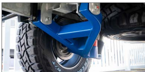
Independent suspension w/ monotube shocks, airbags, disc brakes
