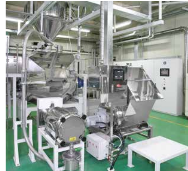
5. Equipment for in-feeding and conveying supplemental materials
