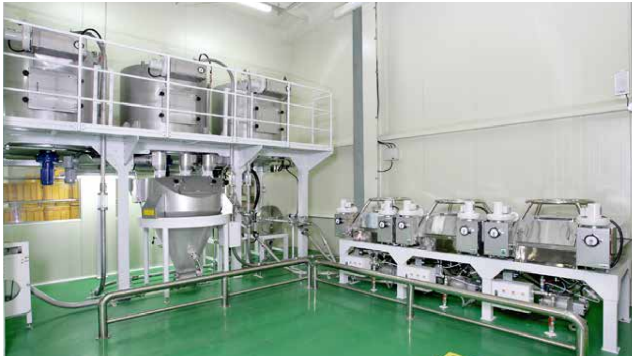
1. Equipment for receiving, milling, storing, weighing and sifting main materials
