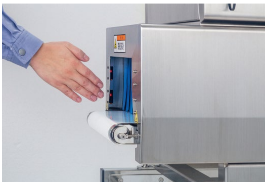
Safety sensors are embedded at access points to provide additional safety.
