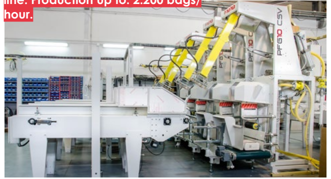
Filling spout and suction cups to hold the empty bag in place.
