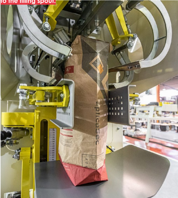
Use the height adjustment to precisely adjust the bag to the filling spout.
