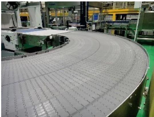
Budweiser Group Beer Conveyor Line - Modular Belt Flat Top Curve Conveyor Project
