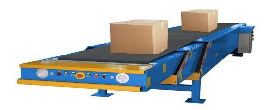
The ICONVEY telescopic belt conveyor is used to realize the functions of fast conveying and loading of items with small footprint and strong applicability. It is composed of multi-layer belt conveyors, which can easily realize the function of conveying items. After unfolding, it can realize long-distance conveying. It is widely used in express/logistics (business site/terminal distribution point), tobacco, chemical industry, food, beverage, alcohol, daily necessities and other industries.
